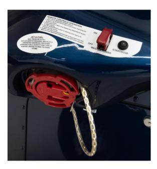
Adding single point fueling capability makes your fuel stops at airports simpler, safer and faster. This modification enables your Caravan to be fueled by standard fueling trucks at ground level removing the requirement for tall ladders and filling tanks individually. Reduce your fueling time so you can get on to your destination faster!
