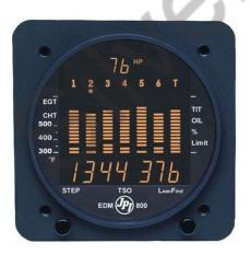
The EDM 800 records, ALL 29 functions, every 6 Seconds, for up to 25hrs., or every minute for 550 hrs., including fuel used. Data downloads to any computer. USB port optional.
