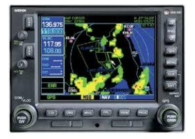
GNS 530 is an all-in-one GPS/Nav/Comm solution. It features a TSO-certified GPS, 2280-channel capacity comm and 200-channel ILS/VOR with localizer and glideslope. Traditionally it would take a host of components to provide the capabilities of this one smart box. High-speed 5 Hz processing makes navigation calculations and map redraw rates five times faster than earlier GNS series navigators.
