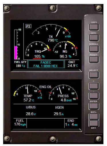
The Vehicle and Engine Multifunction Display (VEMD) and the First Limit Indicator (FLI) both serve to increase the aircraft's safety during flight, reducing the number of gauges that need to be monitored by the pilot. For increased smoothness in flight, which positively affects passenger comfort as well as safety, stability augmentation systems can be installed.
