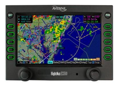
The EX500's user interface dramatically improves your ability to access and display critical flight data. This design philosophy keeps operation simple and consistent by allowing you to select and display what you need on a single easy-to interpret integrated moving map. As a radar display replacement, the EX500 provides easy access to radar modes, tilt control, and bearing adjust.
