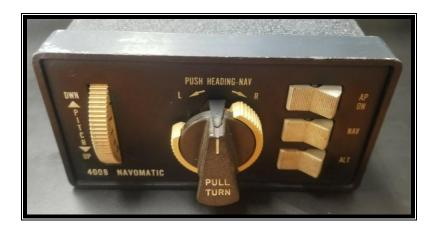
A position-based, two-axis autopilot with full altitude functions including altitude hold and glideslope coupling. The 400B gets heading info from a DG or HSI and can interface to the Flight Director. Auto-trim is standard.
