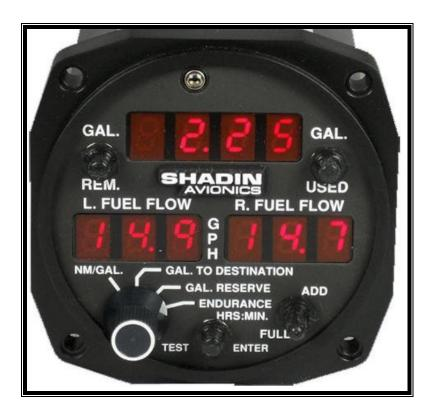
Digiflo-L is a Digital Fuel Management System designed to provide complete fuel management information under real flight conditions without any manual entry of data (after entry of the initial fuel on board information).
