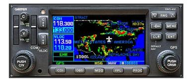
GNS 430 is an all-in-one GPS/Nav/Comm solution. It features a TSO-certified GPS, 2280-channel capacity comm and 200-channel ILS/VOR with localizer and glideslope. Traditionally it would take a host of components to provide the capabilities of this one smart box. High-speed 5 Hz processing makes navigation calculations and map redraw rates five times faster than earlier GNS series navigators.
