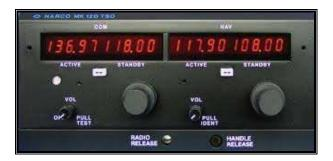
The MK-12D has a bright gas-discharge display, with automatic dimming. This display shows simultaneous active and standby frequencies for both the NAV and COMM sides. The MK-12D NAV/COMM tunes in 200 NAV channels and 720 COMM channels.
